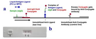
Figure 1 Principle of Pr3/MPO/GBM AI-LFA (a) and AI-LFA cassette (b)
